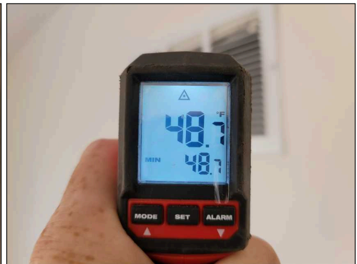
Supply/Air out temperature (48°F)
