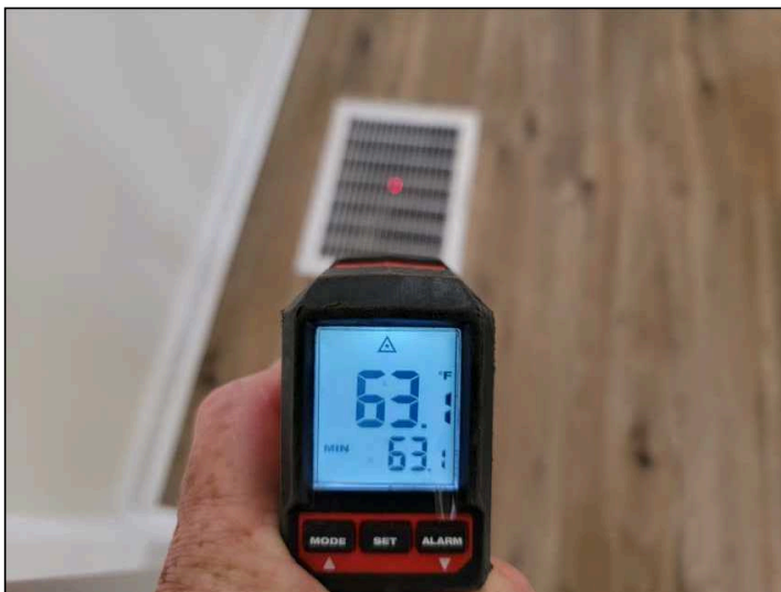
Return/Air in temperature (63°F)
